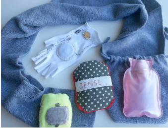
Figure 1: Example of wearable artefacts to be utilised in conjunction with the Focusing technique to interrogate the role of bodily self-awareness in the process of meaning-generation. These props use digital and non-technological means to generate direct sensory stimulation on the body. For instance, we use gloves with vibratory elements, and mini hot water bags to be placed in pouches of different textures. These artefacts and techniques have been previously explored in the workshop Somatic Evaluation Methods developed as part of the Studio component of the Master of Interaction Design and Electronic Arts at the University of Sydney [10].
